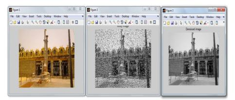
Fig. 5.d. Matlab Results of median filter with filtered and denoised output image in grayscale Fig 5.d shows the Matlab output with real time color image getting converted to grayscale and median filtering on FPGA is performed, as it is very effective in removing the impulsive noise like salt and pepper noise without any blurring of original image.
