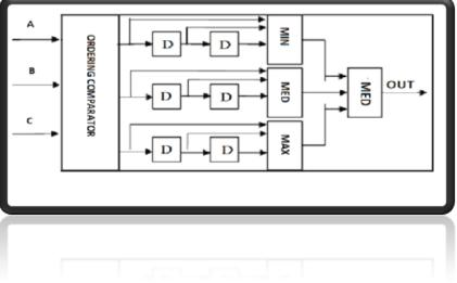
Fig. 4 Hardware module of median filter
