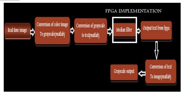
Fig. 3 Block diagram of Image median filtering
