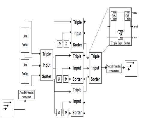
Fig. 2 block diagram of 3x3 triple input sorter based median filter design
